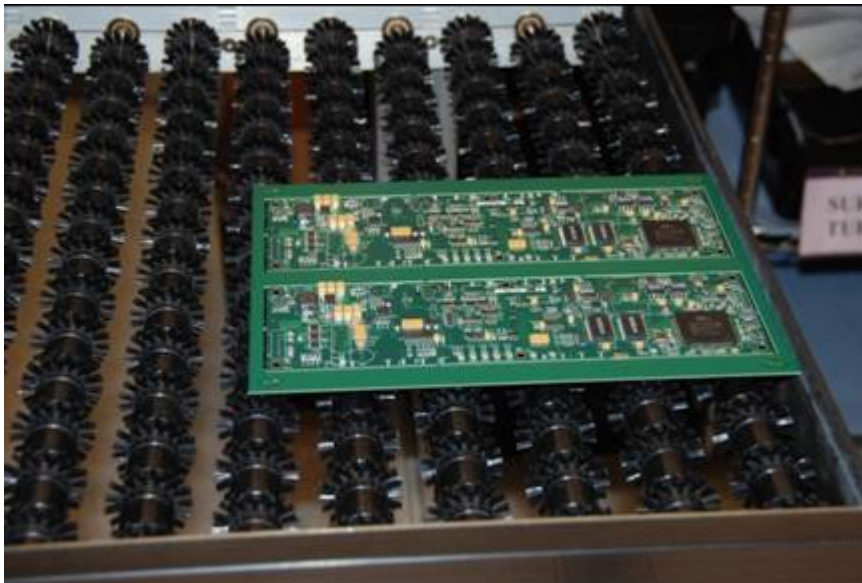
Figure 28: Uncontrolled brushes generate > 500V on PCBs
