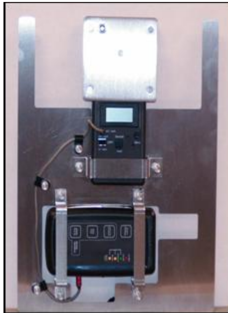
Figure 26: Instrument carrier with portable CPM and recording device
